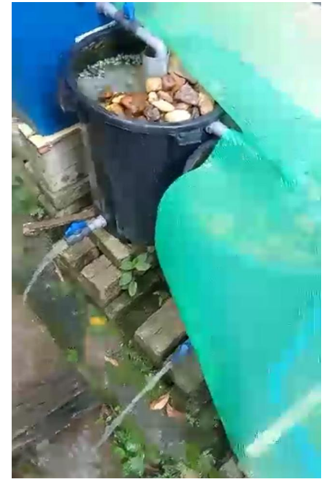
Backwashing up-flow roughing filter
