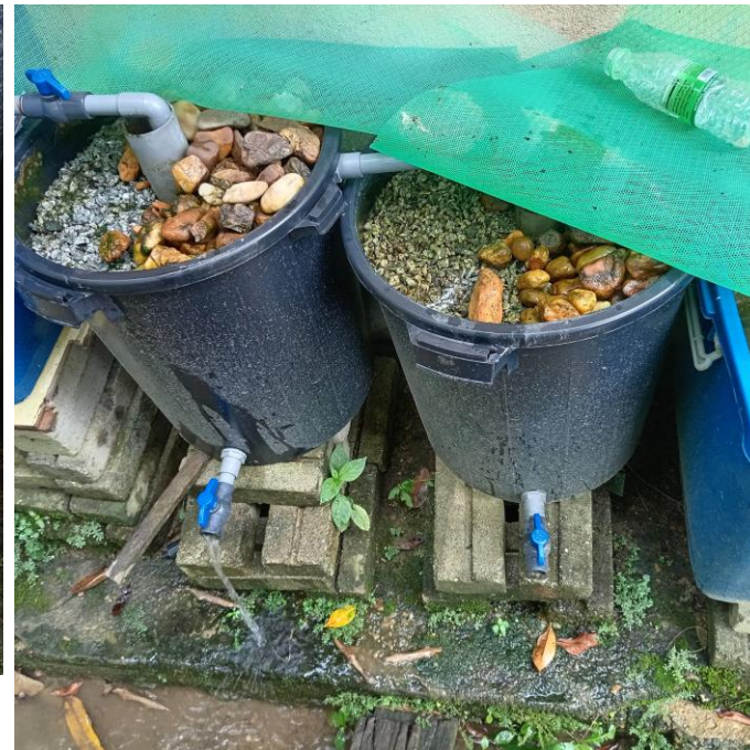
Backwashing up-flow roughing filter
